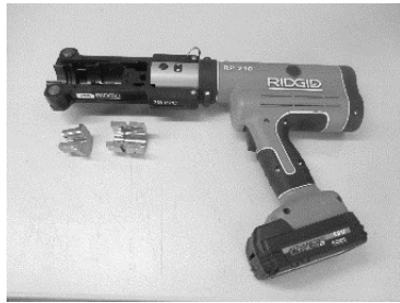
Cold Weld toolset: Rosenberger 11W119-C03/90 inserts with RIDGID tool RP 210/240 and Press Frameset 7/8"
