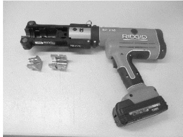
Cold Weld toolset: Rosenberger 11W119-C08/90 inserts with RIDGID tool RP 210/240 and Press Frameset 7/8"
