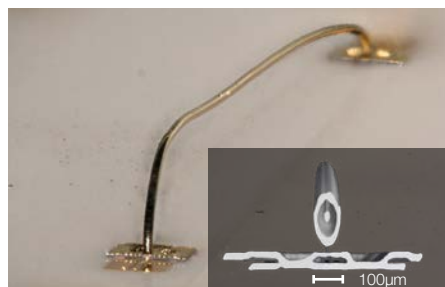
Coax Wire Bond with sectional view
